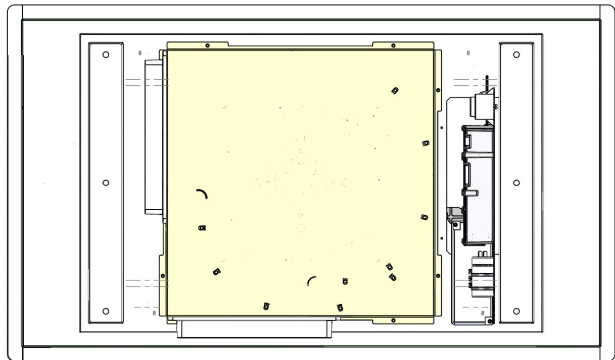
*For the installation, create a false ceiling with a niche of 815mm for 465mm whose minimum height to be reached is 200mm*
